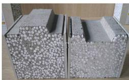
Styrofoam mixed with concrete used in slabs and walls ( reduce the weight of concrete )
