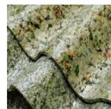
Waste tetrapack used to make roofing
